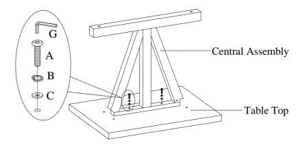
STEP 2: Attach the front/back assembly to table top by using 4 bolts(A), lock washers(B) flat washers(C) and 2 bolts(D), lock washers(E) flat washers(F) as shown below. Completely tighten all bolts. Turn the assembled table to the upright position.
