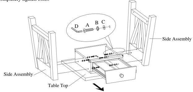
STEP 2: Attach the bottom shelf to side assemblies by using 4 bolts(A), lock washers(B) and flat washers(C). Use the Allen wrench provided to tighten all the bolts. Push back the drawer. Turn the assembled table to the upright position.
