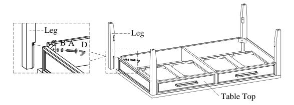
STEP 2: Attach the shelf frame to legs by using 4 bolts(A), lock washers(B), flat washers(C) with an allen wrenchs(D). Completely tighten all bolts. Turn the assembled table to the upright position.
