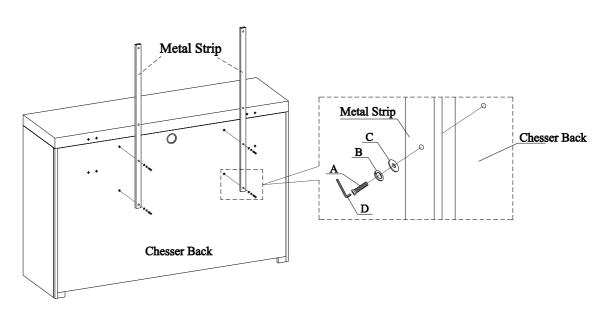
STEP 2: Attach the metal strips to the TV frame by using 4 bolts (A), lock washers (B) and flat washers (C). Tighten all the bolts on TV frame and Chesser with Allen wrench.
