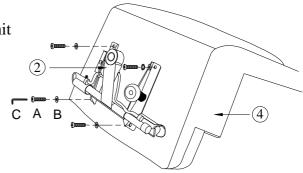
STEP 3: Place the Seating Unit (4) onto the Pneumatic Cylinder (1), aligning the top of the Pneumatic Cylinder (1) to the hole in the Seat Plate (2).
