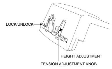
Seat Tilt Tension Adjustment:
