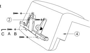
STEP 3: Place the Seating Unit (4) onto the Pneumatic Cylinder (1), aligning the top of the Pneumatic Cylinder (1) to the hole in the Seat Plate (2).
