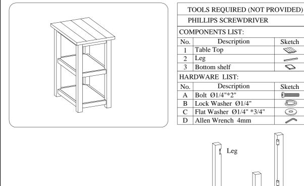
STEP 1: Put the table top face down on a soft surface. Attach the legs to table top by using 4 bolts(A), lock washers(B) and flat washers(C). Do not completely tighten bolts.
