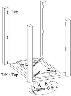
STEP 2: Attach the bottom shelves to legs by using 8 bolts(A), lock washers(B) and flat washers(C). Completely tighten all bolts. Turn the assembled table to the upright position.
