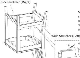
STEP 4: Attach the side stretcher(left) and side stretcher(right) to the front legs and chair back using wood screws(G). Completely tighten all wood screws and bolts. Turn the assembled chair to the upright position.
