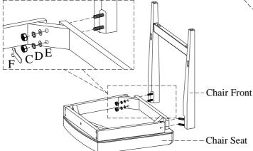
STEP 2: Attach the assembled chair front to chair seat by using 4 flat washers(E), lock washers(D), and hex nuts(C) with a hex wrench(F), Do not tighten bolts until STEP 4.
