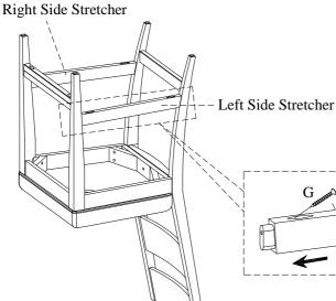
STEP 4: Attach the left side stretcher and right side stretcher to the front legs and chair back with wood screws(G). Completely tighten all wood screws and bolts. Turn the assembled chair to the upright position.
