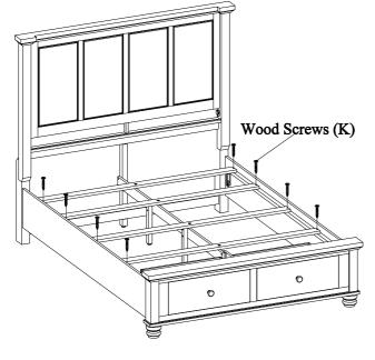
STEP 8: Arrange slats on the slat bearers and then lay decking on top of the slats. Make sure the slats are positioned along the seams of the decking as shown in the detail in STEP 9 under the pre-drilled hole. Remove the decking and attach slats to the slat bearers with wood screws (K).
