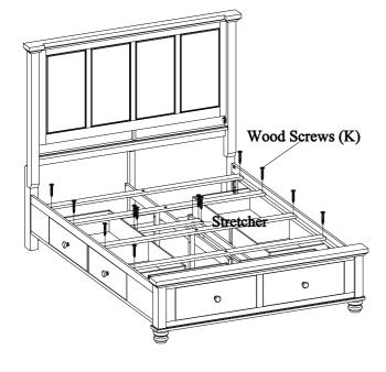
STEP 9: Attach the stretcher to side storage rails on both sides and Arrange slats on the slat bearers and then lay decking on top of the slats. Make sure the slats are positioned along the seams of the decking as shown in the detail in STEP 10 under the pre-drilled hole. Remove the decking and attach slats to the slat bearers with wood screws (K).
