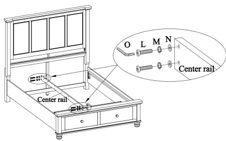
STEP 7: Attach 2 support legs (for center rail) to the center rail using 4 bolts(L), lock washers(M) and flat washers(N). Use the Allen Wrench (O) to tighten all of the bolts.
