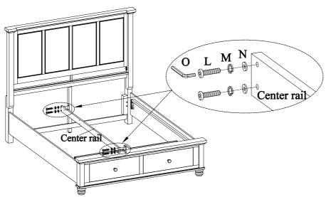
STEP 7: Attach 2 support legs (for center rail) to the center rail using 4 bolts(L), lock washers(M) and flat washers(N). Use the Allen Wrench (O) to tighten all of the bolts.
