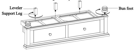
STEP 5: Put side storage rails upside down on a padded, clean surface. Attach support legs (for side storage rail) to footboard. Turn side storage rails right side up.
