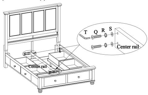
STEP 9: Attach 2 support legs (for center rail) to the center rail using 4 bolts(Q), lock washers(R) and flat washers(S). Use the Allen Wrench (T) to tighten all of the bolts.
