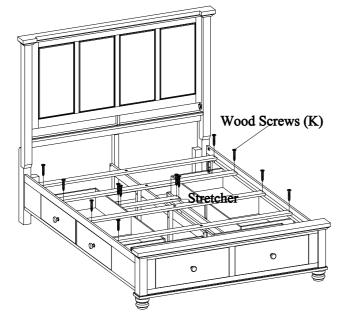
STEP 10: Attach the stretcher to side storage rails on both sides and Arrange slats on the slat bearers and then lay decking on top of the slats. Make sure the slats are positioned along the seams of the decking as shown in the detail in STEP 11 under the pre-drilled hole. Remove the decking and attach slats to the slat bearers with wood screws (K).
