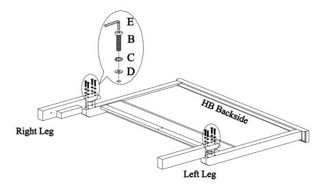
STEP 2: Attach the wood stretcher to the legs by using 2 bolts(A), lock washers(C) and flat washers(D).
