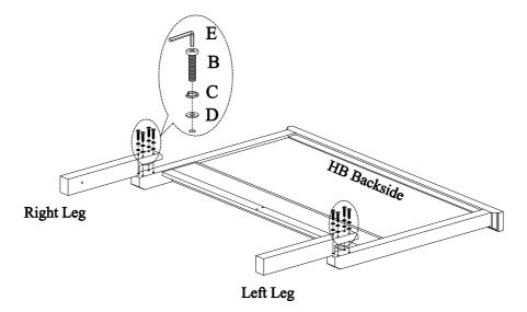
STEP 2: Attach the wood stretcher to the legs by using 2 bolts(A), lock washers(C) and flat washers(D).
