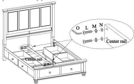
STEP 8: Attach 2 support legs (for center rail) to the center rail using 4 bolts(L), lock washers(M) and flat washers(N). Use the Allen Wrench (O) to tighten all of the bolts.
