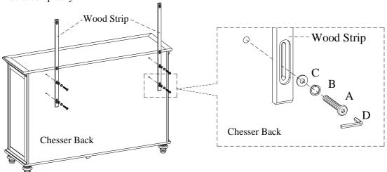
STEP 2: Attach the wood strips to the mirror by using 4 bolts(A), lock washers(B), and flat washers(C). Tighten all bolts on Chesser and mirror with Allen wrench.
