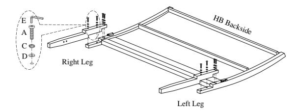
STEP 2: Attach the wood stretcher to the legs by using 4 bolts (B), lock washers (C) and flat washers (D). Use the Allen wrench (E) provided to tighten all the bolts.
