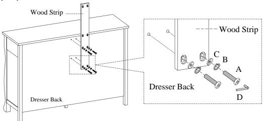
STEP 2: Attach the wood strip to the mirror by using 4 bolts(A), lock washers(B), and flat washers(C). Tighten all bolts on dresser and mirror with Allen wrench.
