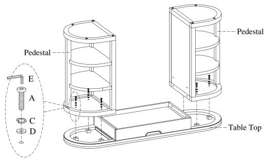
STEP 2: Pull out the flip down keyboard drawer, then attach "U" shape frame with both pedestals by using 8 bolts(B), lock washers(C) and flat washers(D) as shown below. Use the Allen wrench provided to tighten all the bolts. Push back the flip down keyboard drawer. Turn the assembled table to the upright position.
