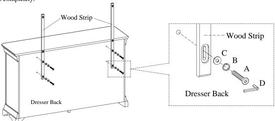
STEP 2: Attach the wood strips to the mirror by using 4 bolts(A), lock washers(B), and flat washers(C). Tighten all bolts on dresser and mirror with Allen wrench.
