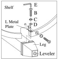
STEP 1: Attach the legs to the shelves by using 12 bolts(B), lock washers(C) and flat washers(D) with 6 L metal plates.
