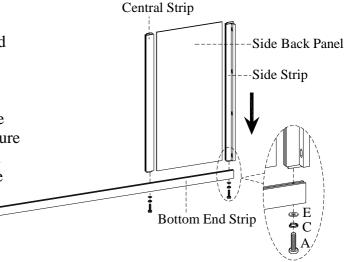
STEP 2: Then insert the central back panel with the cord hole in the bottom. Attach the top end strip to whole back panel using 4 bolts(A), lock washers(C) and flat washers(E). Make sure the back panels' finished side is facing inward. Completely tighten all bolts.
