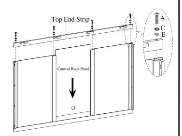
STEP 3: Attach the back panel assembly to the left pedestal and right pedestal using 8 bolts (B), lock washers (C) and flat washers (D). Do not tighten bolts until STEP 4.
