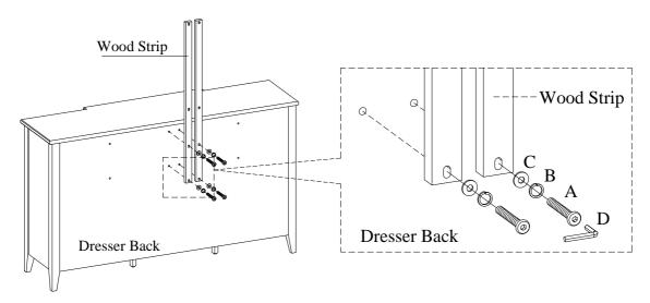
STEP 2: Attach the wood strips to the mirror by using 4 bolts(A), lock washers(B), and flat washers(C). Tighten all bolts on dresser and mirror with an allen wrench(D).
