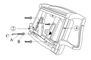
STEP 3: Place the Seating Unit(4) onto the Pneumatic Cylinder(1), aligning the top of the Pneumatic Cylinder(1) to the hole in the Seating Plate(2).
