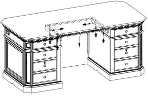
STEP 2: Attach Typical Swivel Keyboard to Mounting Plate by using 4 bolts, lock washers, flat washers and nuts. Using open wrench tighten all these bolts. (This hardware is included with Keyboard)
