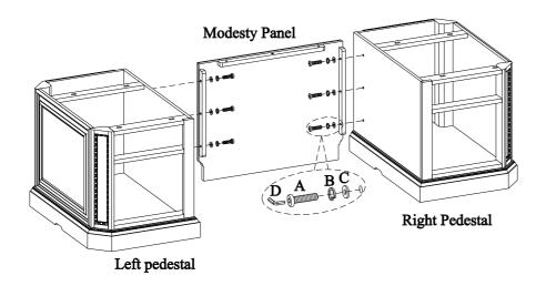
STEP 3: Attach the pedestals and modesty panel to the desk top by using 11 bolts(A), lock washers(B), flat washers(C). Completely tighten all bolts used in Steps 2 and 3.
