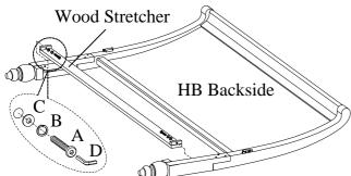
STEP 2: Attach the wood stretcher to the legs by using 2 bolts(A), lock washers(B) and flat washers(C).
