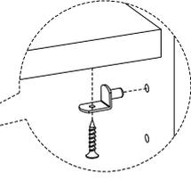
If you prefer to adjust the shelf location, remove the screws and move shelf brackets to the desired location. Then secure the brackets to shelf with screws.
