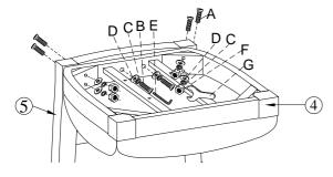
STEP 2: Attach Seating (4) to Chair back (5) by using bolts (A), bolts (B), lock washer (C), and flat washer (D), use Allen key (E) and hex wrench (G) tighten all bolts.
