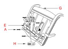
3.Insert the Seating Unit (G)onto the Pneumatic Cylinder(D).
